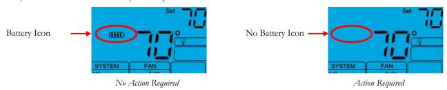
**Remedy:** Customers with a 1F8X-04XX thermostat that **does not** show a battery icon **to** on the thermostat screen should contact White-Rodgers for assistance with the corrective action or visit the White-Rodgers website. For affected thermostats, a packet will be sent which includes instructions on the corrective action.
